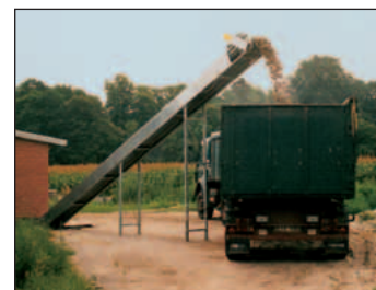
Manure is loaded directly on trucks
