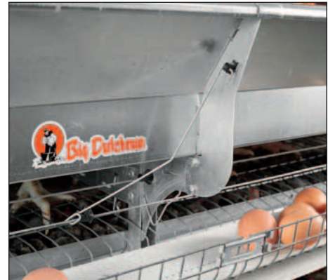
Raised EggSaver makes way for the eggs to roll on to the egg belt
