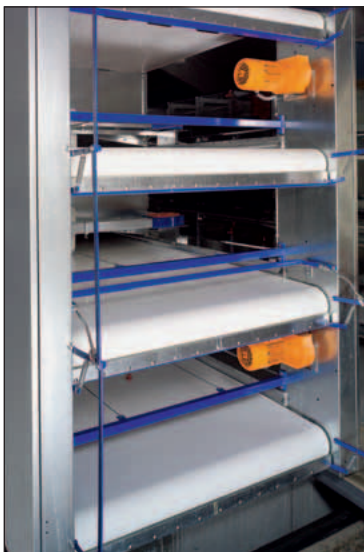
Manure removal end-set with manure chute
